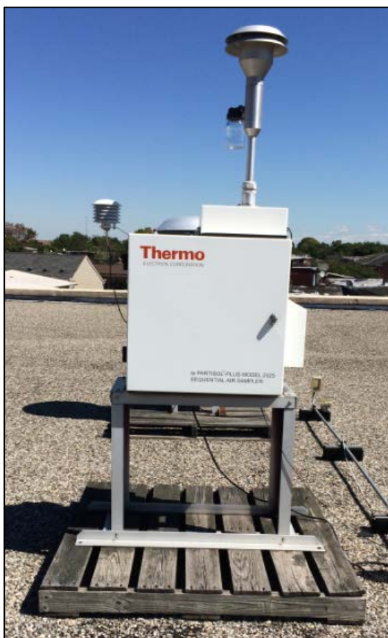
Figure 2-2 USEPA-Approved PM 2.5 Sampler in Trenton
